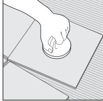
During the installation of the tiles, it is essential that excess setting materials are removed, both on the face of the tile and in the grout joint.
