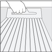
Periodically check back of tile to ensure proper transfer for interior applications — minimum 80% coverage. For exterior, wet, or plywood applications — minimum 95% coverage. For Stone the minimum coverage is 95% with no voids exceeding 2 square inches and no voids within 2" of the corners. Coverage is defined as the area the mortar makes contact with the tile and substrate.
