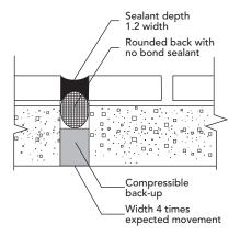
Large areas of tile also need expansion or control joints every 20' - 25' or if in direct sunlight 8' - 12'. Note: exterior installation control joints are set at 8' - 12'.
