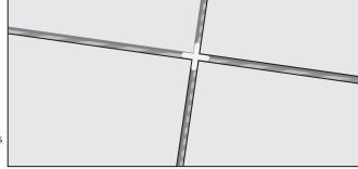
Spacers are generally used to set the width of the grout lines and keep the tiles spacing even.
