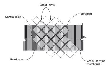
It is a frequent misconception that anti-fracture membranes allow you to eliminate movement joints - they do not. There always must be soft joints in the tilework to allow for expansion and contraction.
