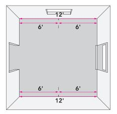
Connect the midpoint marks using a chalk line to find the room's center.
