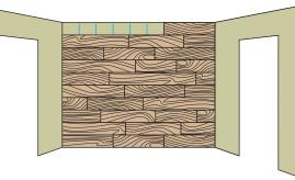
• The last row will need to be cut lengthwise (ripped down) to fit properly to the ceiling, leaving a minimum 1/2" for expansion.
