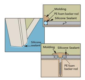
To ensure the floor is able to "float" freely, be sure to affix baseboards or moldings to the walls, not to the floors. This way, the floor can expand & contract within the gap.
