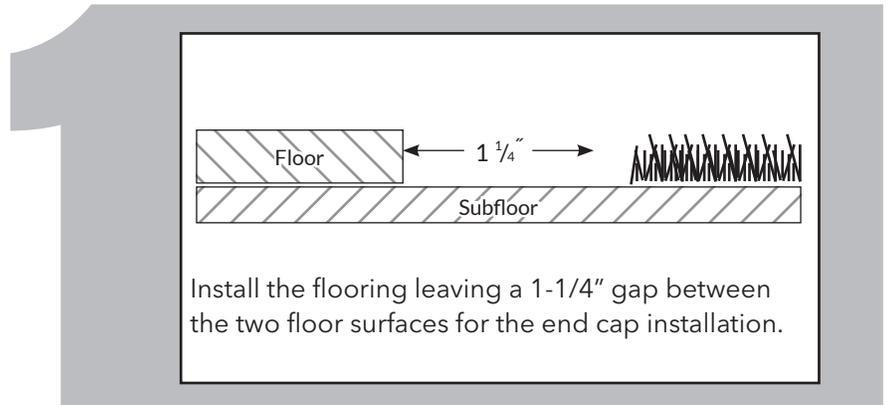
Install the flooring leaving a 1-1/4" gap between the two floor surfaces for the end cap installation.
