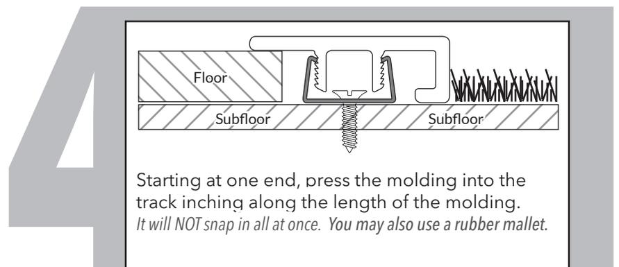
Starting at one end, press the molding into the track inching along the length of the molding. It will NOT snap in all at once. You may also use a rubber mallet.
