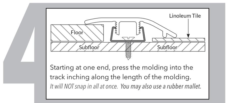
Starting at one end, press the molding into the track inching along the length of the molding. It will NOT snap in all at once. You may also use a rubber mallet.
