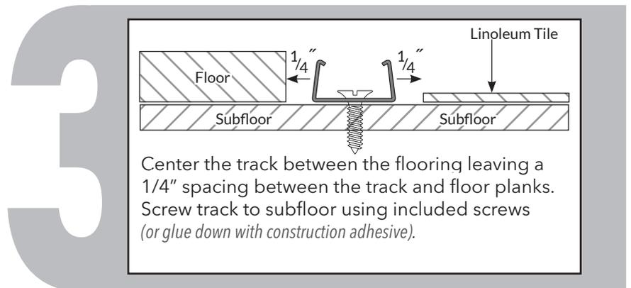
Center the track between the flooring leaving a 1/4" spacing between the track and floor planks. Screw track to subfloor using included screws (or glue down with construction adhesive).
