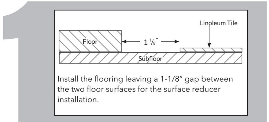
Install the flooring leaving a 1-1/8" gap between the two floor surfaces for the surface reducer installation.
