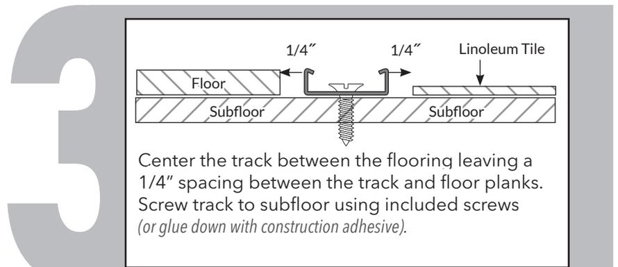
Center the track between the flooring leaving a 1/4" spacing between the track and floor planks. Screw track to subfloor using included screws (or glue down with construction adhesive).
