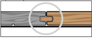
Splines should always be glued into place using a Tongue and Groove adhesive
