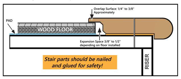
If there is an existing "overhanging" stair nosing, you must cut it off before installing the overlap stair nosing. Trim off to the riser line as shown below:
