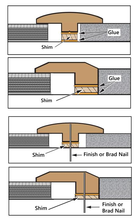
Tip: For best results, pre-glue shim to bottom of transition before installing.
