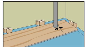
If there are multiple or larger pipes passing through the floor make hole(s) on the plank 1" greater than the diameter of the pipe, cut the plank with a 45° angle towards the hole. The cut-off piece edges are glued in the position again. *Do not glue to the subfloor.*
