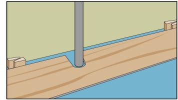
When there is single pipe on a wall, you can plan to have the end-joints meet at pipe, drill and install as shown.
