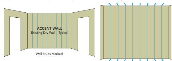
• Using a chalk line stretched between bottom and top mark, snap a line. Use painters tape at top & bottom of **each** stud on floor and ceiling to identify nailing points.
