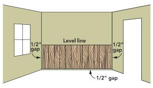
Trim out walls using 3/4" round (avoid nailing into planks).
