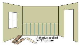
• Set plank in place with the top of the plank on the chalk line leaving a minimum 1/2" expansion space at bottom of wall.
