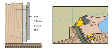
Use a level to double-check the levelness of the line between the two marks. Adjust line as needed with spacers. Secure this first row fully using adhesive and 2' finish nails or wood screws into pre-marked wall studs, placed approximately 2" above subfloor (these will be covered by your baseboard trim).
