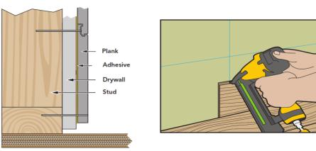
Use a level to double-check the levelness of the line between the two marks. Adjust line as needed with spacers. Secure this first row fully using adhesive and 2' finish nails or wood screws into pre-marked wall studs, placed approximately 2" above subfloor (these will be covered by your baseboard trim).
