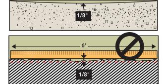
Improper substrate or flatness can result in gaps, locking mechanism failure and premature wear on surface.
