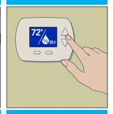
**Maintain** Environment Interior temperature should be maintained between 50°F – 85°F and 30% – 70% Relative Humidity during the life of the floor.
