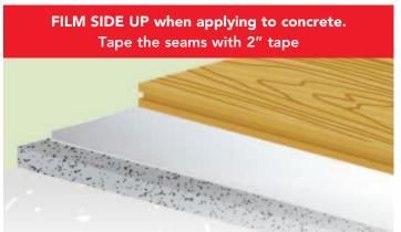
Film side up when applying to concrete to block the moisture from concrete subfloor that could damage the flooring.
