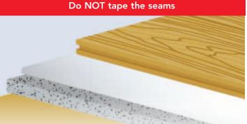
FILM SIDE UP when applying to wood subfloor.
