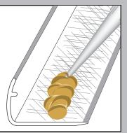
Carefully roll the stair nose against the front of the step, making sure the transition is in place. Once in its desired position, press down firmly over the entire stair nose.
