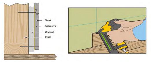
Use a level to double-check the levelness of the line between the two marks. Adjust line as needed with spacers. Secure this first row fully using adhesive and 2' finish nails or wood screws into pre-marked wall studs, placed approximately 2" above subfloor (these will be covered by your baseboard trim).
