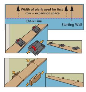
Tip: Scrap flooring (cut up in short strips) may be used for additional spacing material.
