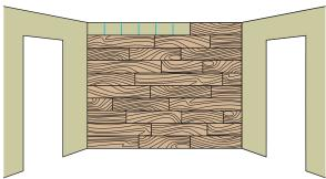
• The last row will need to be cut lengthwise (ripped down) to fit properly to the ceiling, leaving a minimum 1/2" for expansion.
