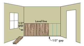
• The last row will need to be cut lengthwise to fit properly, leaving a 1/2" for expansion.
