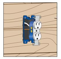
Do not cover receptacle retaining screw /surrounding fixture, to allow for bringing receptacle forward to accommodate for the thickness of new planks.
