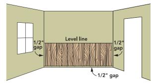
Trim out walls using 3/4" round (avoid nailing into planks). Install baseboard to cover gap along floor and Install threshold along top edge to finish wainscot wall.
