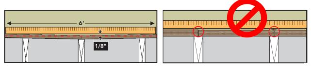
Improper substrate or flatness can result in gaps, squeaks, premature wear on surface and poor plank fitting during assembly.
