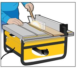
If width of last plank is less than 2.5", balance by cutting (Rip) starting row of planks accordingly.
