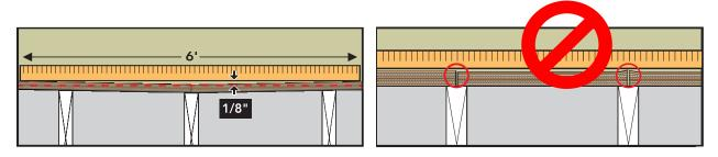
Improper substrate or flatness can result in gaps, squeaks, premature wear on surface and poor plank fitting during assembly.
