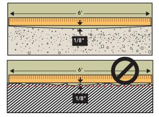
Improper substrate or flatness can result in gaps, locking mechanism failure and premature wear on surface.
