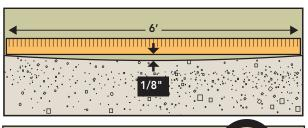
Improper substrate or flatness can result in gaps, locking mechanism failure and premature wear on surface. Correct any issues.
