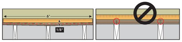
• Improper substrate or flatness can result in gaps, squeaks, premature wear on surface and poor plank fitting during assembly.
