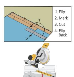
Floor cutters\*, power table, circular and jig saws can also be used to cut this flooring product.
