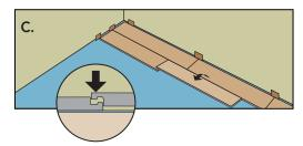
Depending on the length of plank, tap along length of plank as shown to fully engage planks. Ensure tapping block abuts side of plank properly to prevent damage to product face or locking system.
