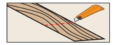
Floor cutters\*, power miter saw, table, circular and jig saws can also be used to cut this flooring product.
